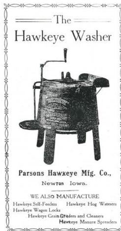
attached at the top. This shaft is formed into a crank at the top end, and to this crank is attached a rack bar which meshes with a cog wheel on the dolly shaft. This gives the dolly, or clothes agitator, the motion inside the tub. A fly wheel is placed on the tub underneath, mounted on ball bearings and driven at high speed by a straight spur gear on the lower end of the crank shaft. This gear is covered with a shield, neatly formed into a soap box.
